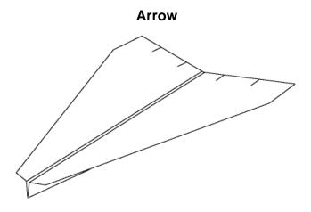
This plane is easy to fold and flies straight and smooth. Add a small amount of up elevator for long level flights.
